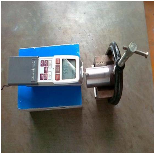
Fig.2. Testing With the help of Roughness Tester
